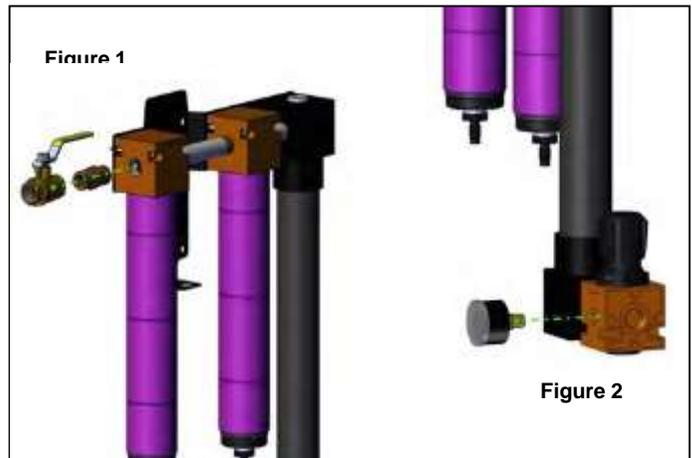
1. Mount the dryer in an upright position. Mount on sturdy wall or frame using the supplied mounting brackets. *Note: If using dryer in an automotive application, install outside of spray booth. Bake cycles may cause premature aging of the membrane inside the unit.*
