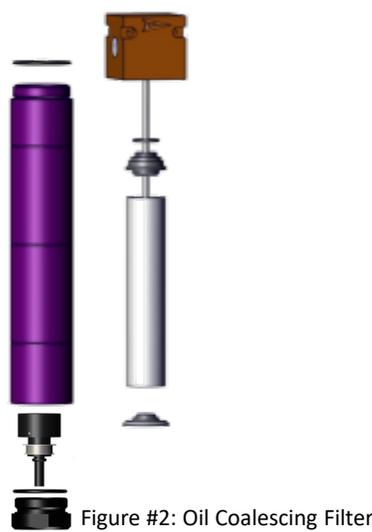
Figure #2: Oil Coalescing Filter
