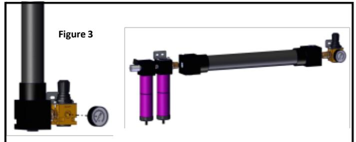
5. Replace Regulator in open port. Be sure to follow flow descriptions on membrane dryer.
